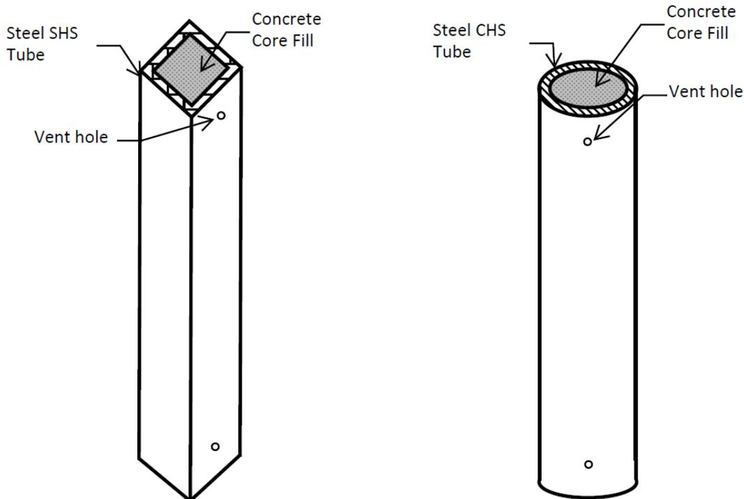
Figure 1. – A typical concrete core-filling detail.
